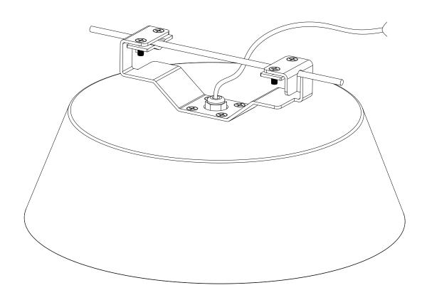
**Notes:** Do not energize luminaire until installation is completed. General contractor is responsible for providing appropriate anchoring devices to support load of fixture.
